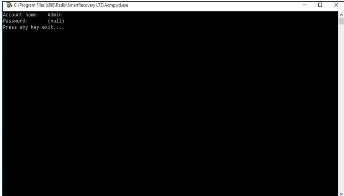
Figure 4-1: Password recovery screen. Note that the password is (null), since the password is presently blank.
